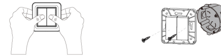
①Put in the middle to take off the key frame ②Fix the back cover of the switch to the switch box or the expansion rubber
